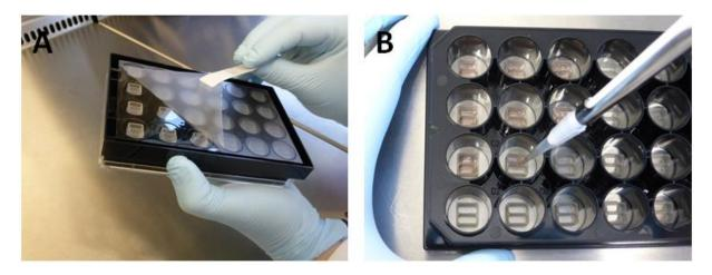
Figure 2 Remove the protective foil before starting the cell seeding step (A). Fill 70  $\mu$ l of cell suspension into each well of the Culture-Inserts 2 Well (B).
