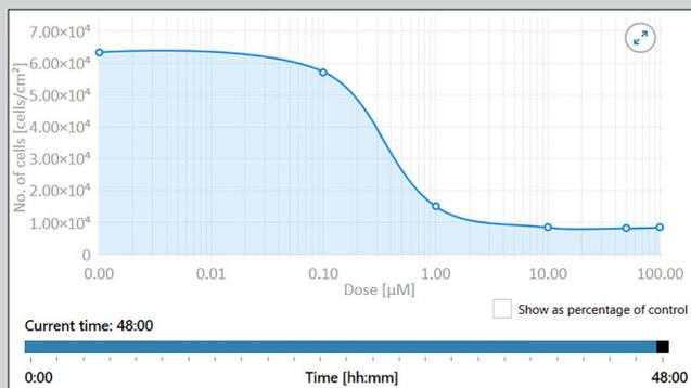
The HoloMonitor Kinetic Dose Response Assay automatically provides interactive *in vitro* dose response curves at any time point.
